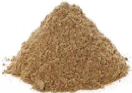
Fine aggregate are the materials passing through IS sieve that is less than 4.75 mm sieve. Usually natural sand is used as a fine aggregate due to scarcity crushed stone is used in this project.
