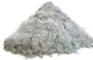
Fly ash is a fine, powdery material that is a byproduct of burning pulverized coal in thermal power plants. Fly ash primarily consists of silica, alumina, and iron, and possesses pozzolanic properties, meaning it can react with calcium hydroxide in the presence of water to form compounds with cementitious properties, that cement was partially replaced with fly ash at 30%.
