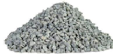
Coarse aggregate are the materials retained on 4.75 mm sieve and the broken stone is generally used. According to IS 383:1970 maximum 20 mm coarse aggregate is suitable for concrete. The nature of work decides the maximum size of coarse aggregate.
