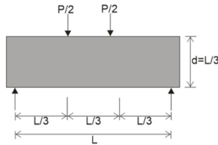
Fig. 3. Third-Point Load Test Setup.
