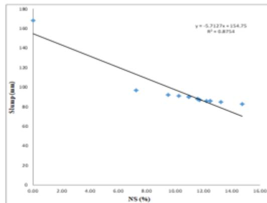
**Fig. 7. Control Mixes Result of Slump Test on Nano-silica Blended Concrete**
