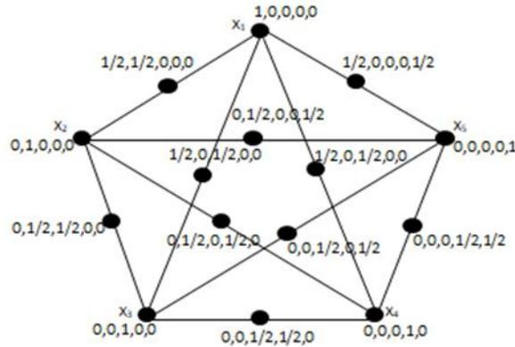
Fig.2: A Factor Space for a 5-Component Concrete Mixture used in this Study
