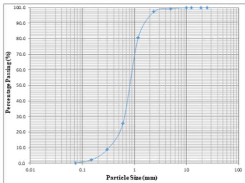
Fig. 4. Chart of Particle Size Distribution for Sand
