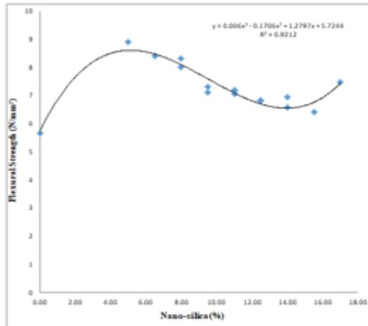
Fig. 8. Result of Flexural Strength of Hardened Nano-silica Blended Concrete Beam Specimens of Trial Mixes at 28 Days
