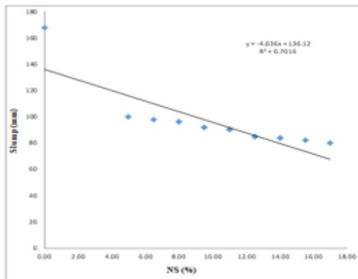
**Fig. 6. Trial Mixes Result of Slump Test on Fresh Nano-silica Blended Concrete**
