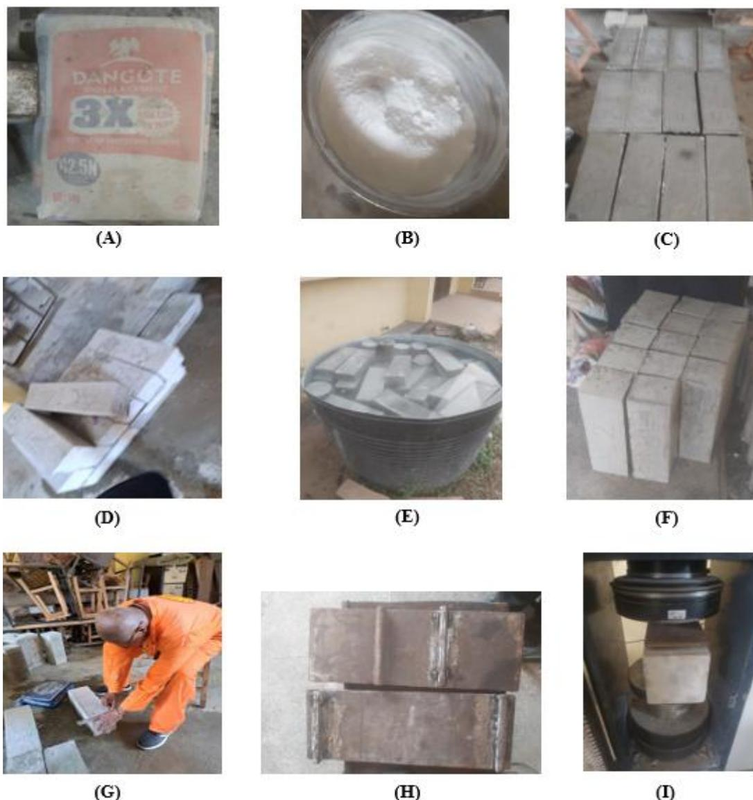
**Fig. 1:** (A) Portland Limestone Cement (B) NS (C) NSB Concrete in Beam Moulds (D) Demoulded NSB Concrete Beam Specimens (E) NS Beam Specimens in Curing Tank (F) NSB Concrete Beam Specimens to be Marked for Testing (G) Marking of NSB Concrete Beam Specimens for Flexural Test (H) Support Mechanism for Third Point Load Test (I) Third Point Load Test on NSB Concrete Beam Specimen
