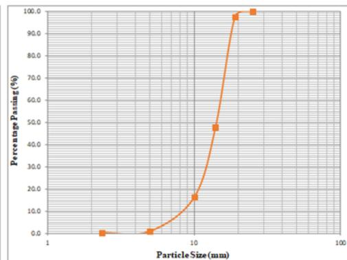
Fig. 5. Chart of Particle Size Distribution Curve for Granite
