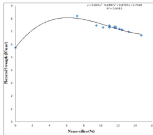
Fig. 9. Result of Flexural Strength of Hardened Nano-silica Blended Concrete Beam Specimens of Control Mixes at 28 Days
