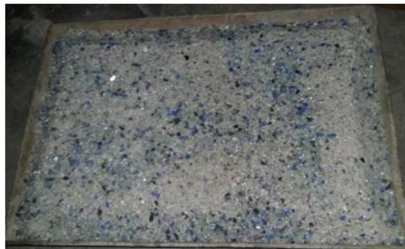
**Figure 1:** Crushed waste glass
