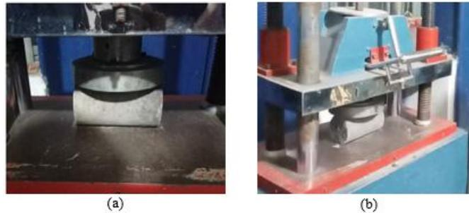
Figure 4: (a) Before crushing & (b) After crushing of cylinder specimens
