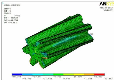
Fig : Stress Plot For Helical Gears
