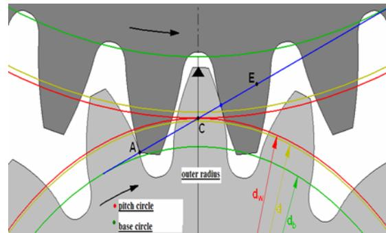
Fig 10: Interference in Gears
