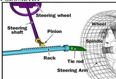
Fig 8: Rack and Pinion in steering
