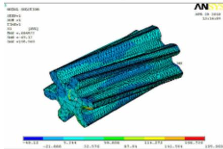
Fig : Displacement Results For Helical Gears
