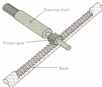
Fig 7: Rack and Pinion
