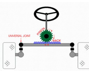
Fig 9: Rack and Pinion arrangement
