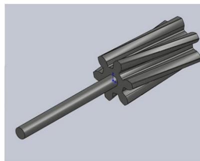
Fig 14: CAD Model of Helical Gear Pinion
