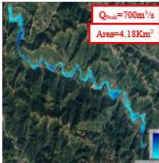
Figure 2-5 Flood Inundation Map after dam breaching for inflow of 700 cumecs.
