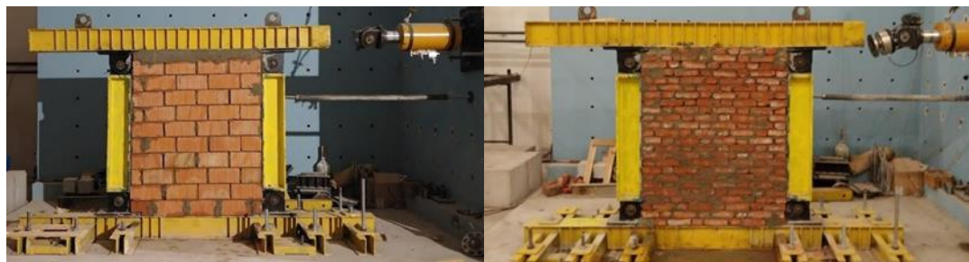
(a) wall made of vertical perforated bricks (b) Threshing bricks wall Figure 3. Constitutive Sample of Masonry Walls inside a steel frame
