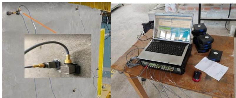
Figure 5. accelerometers placed on the wall and B&K type 3560-C data collection unit
