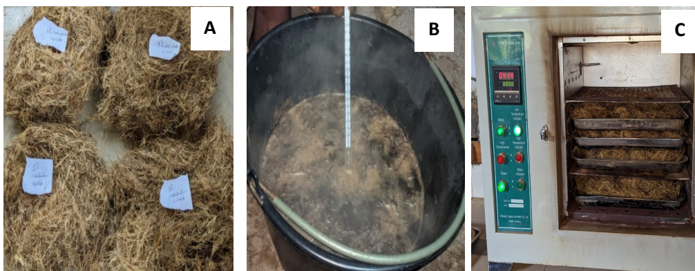
Figure 3: Extracted EFBSF and CF(A) Pretreating fibres (B) Oven drying of treated fibres(C)
