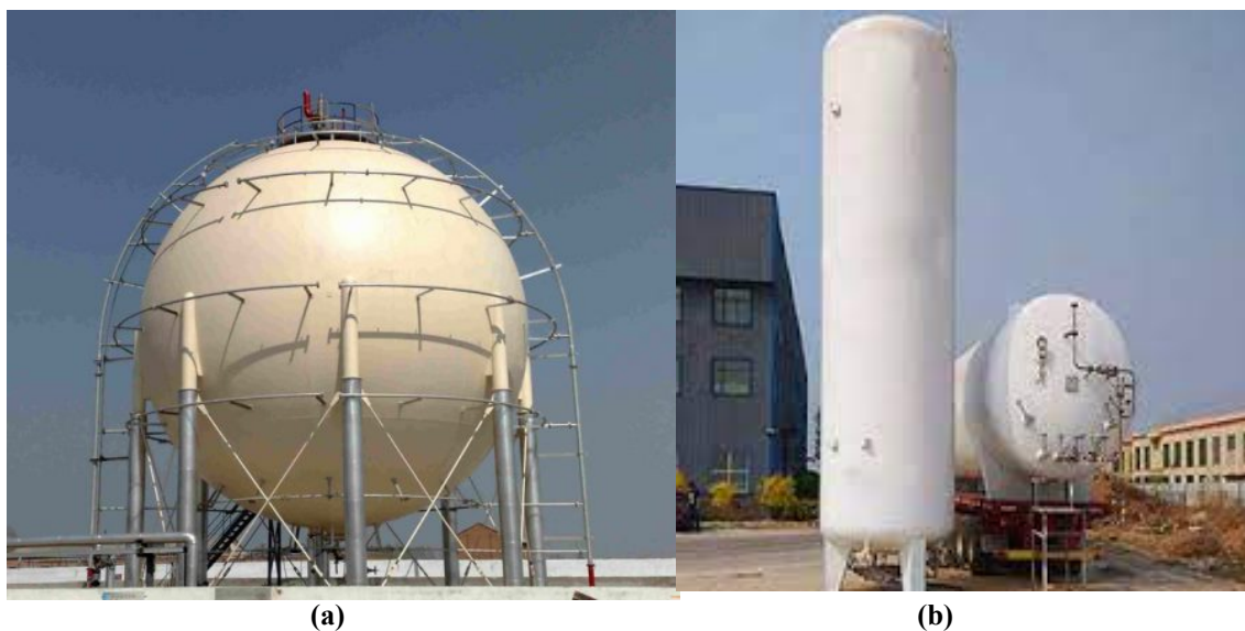
Fig 1.1: Spherical (a) and Cylindrical (b) Pressure Vessels.
