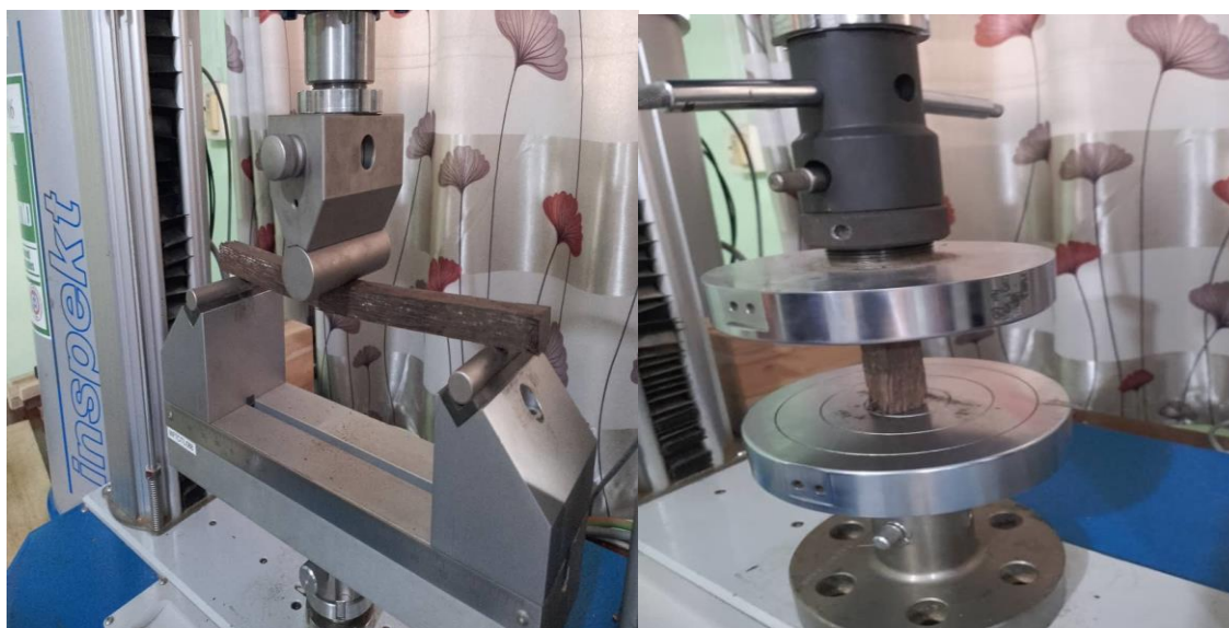
(a) Three-point bending test (b) Compression test Figure 4: Three-point bending and compression test set-up
