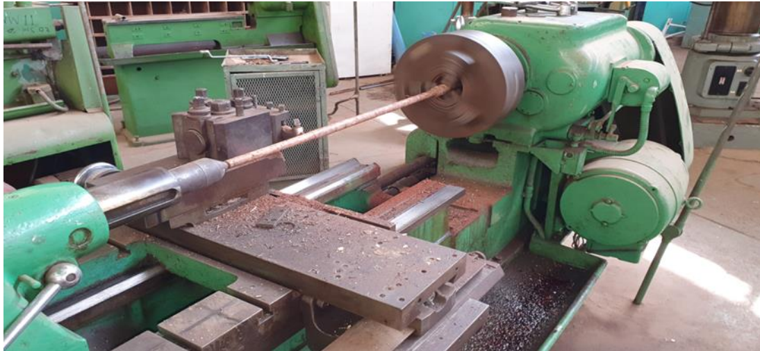
(a) Fan palm bar being prepared on a lathe machine
