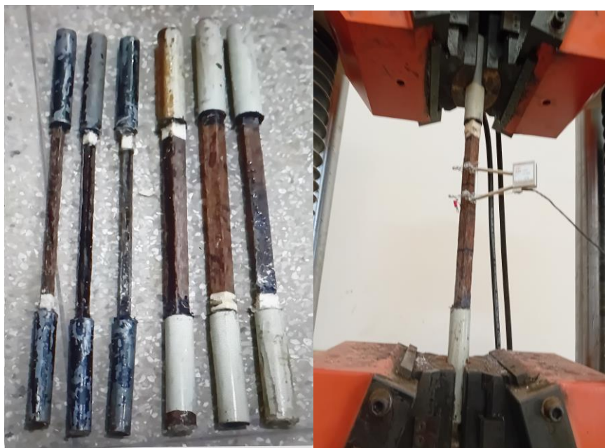
(a) Grip enhancement mechanism (b) extensometer attached to the fan palm bar Figure 3: (a) Sample specimens and (b) Specimen clamped into the UTM
