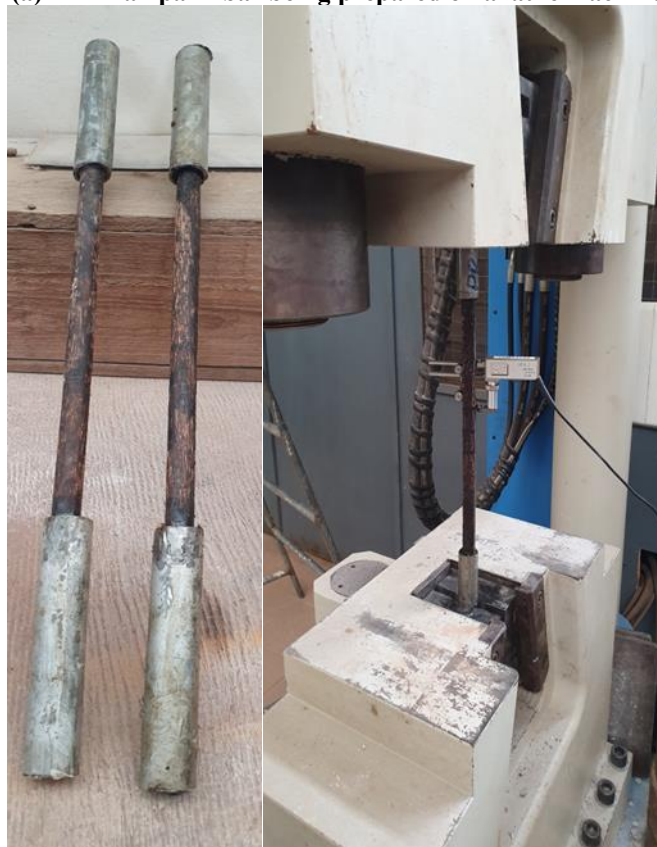
(b) fan palm bar grip (c) specimen for a tensile pull using UTM Figure 5: Preparations of specimen for the Poisson ratio test using UTM
