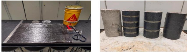
Figure 2: Preparation and application of Carbon Fibre Reinforced Polymer (CFRP) composites on concrete columns.
