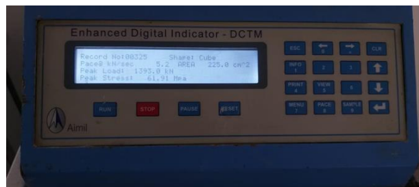
Figure 1: Cube strength test with CNTs 0.2% weight of cement with Average result Value 60 Mpa after 28 days.
