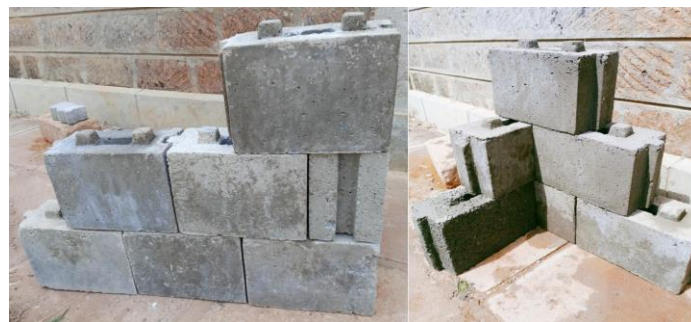
Figure 6: A pictorial representation of how the hollow interlocking blocks made using the mold interlock at the corners
