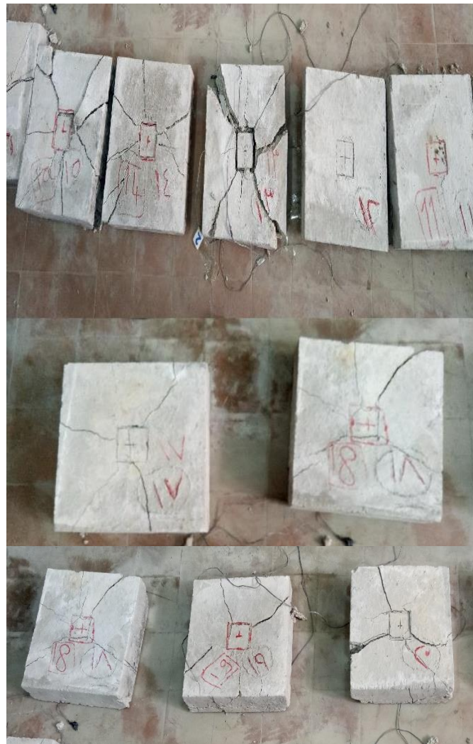
Fig. (12) Failure of some tested specimens
