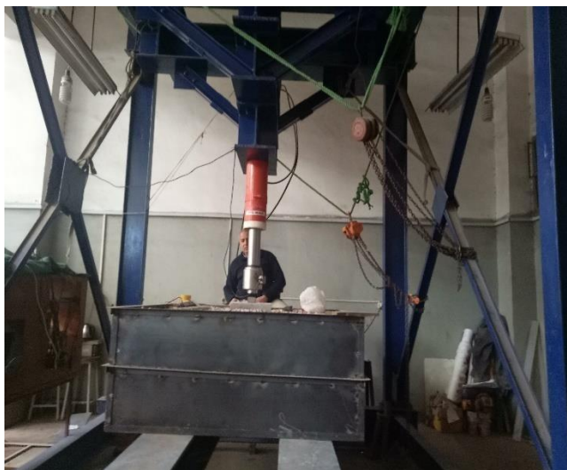
Fig (10) Steel Container and loading frame
