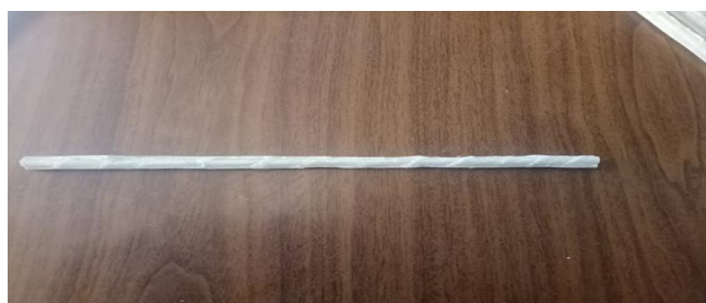
Fig (2) Fiber carbon bars (CFRPs)
