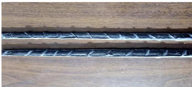
Fig (1) Fiber glass bars (GFRPs)
