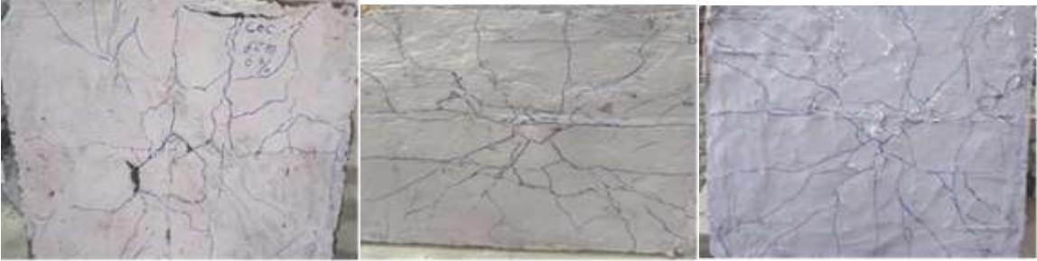
Fig 6: crack pattern of the tested slabs for group (1).
