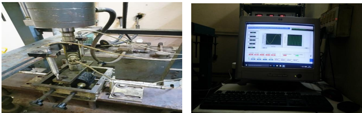
Figure 3: Specimen arrangement for Indirect Tensile Fatigue test
