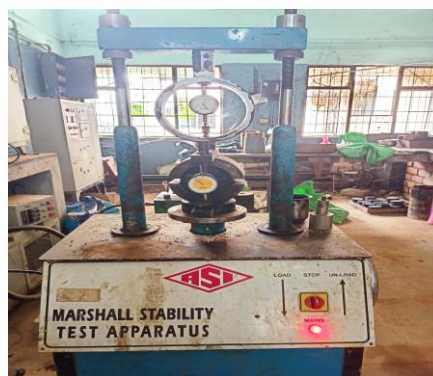
Figure 1: Specimen arrangement for marshall stability test
