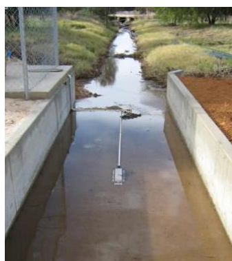
Figure 5. Canal discharge measurement telemetry system
