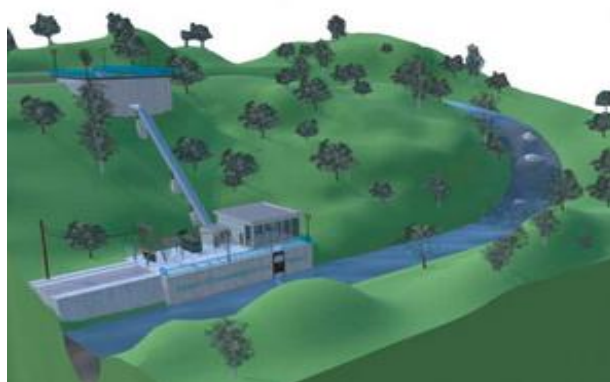
Figure 8. Typical run-of-river hydropower schemes
