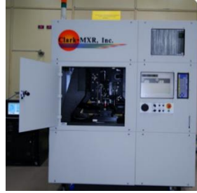
Fig-2: Femtosecond laser Micro Machining System at CMTI
