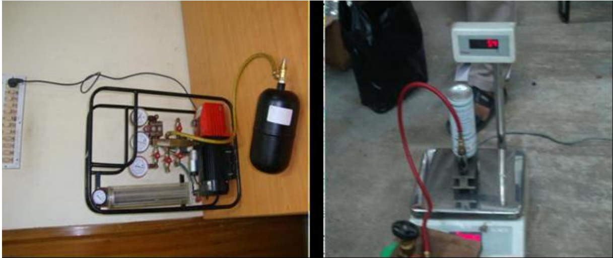
Fig no 2.2 Shows the charging setup of refrigerants by mass proportion
