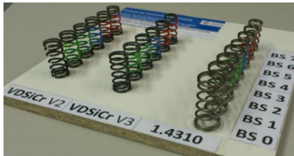
Figure 2. Picture of springs with code names used in FE analyses and material codes
