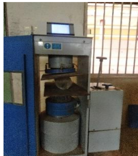
Figure 4: Compression machine for tensile strength test
