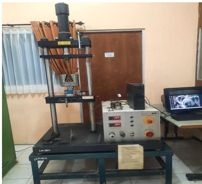
Figure 2. Tensile Testing Equipment Model WP 310 Gunt Hamburg Material Testing Machine
