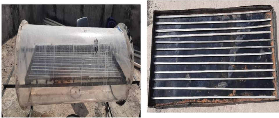
Figure 1. Photographic view of Tubular solar still equipped with mica sheet and aluminium fins.
