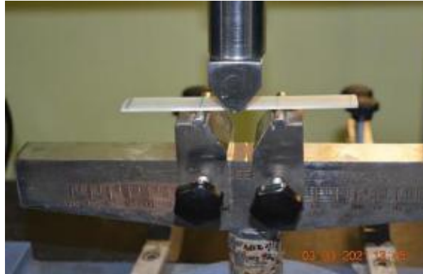
Fig.9: Three point bending fixture
