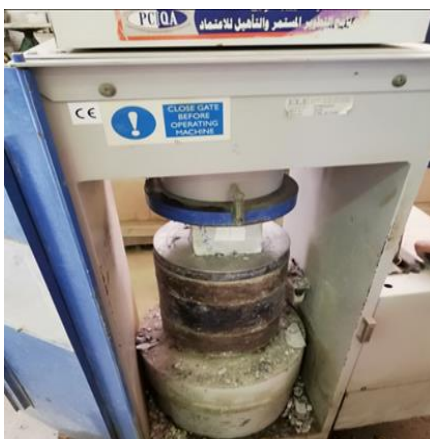
Fig. 4: Cube (10 × 10 ×10 cm) during Compressive Strength test
