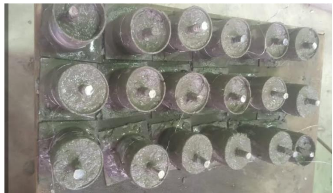
Fig. 4: Cylinders (70 ×100 mm) During Casting
