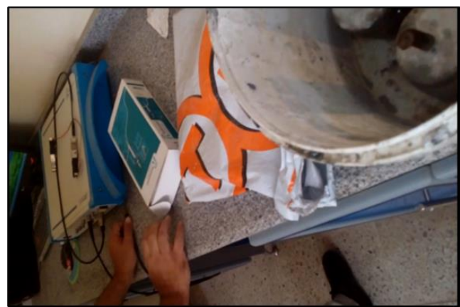
Fig. 5: Cylinder (7 × 10 cm) During Measuring Corrosion
