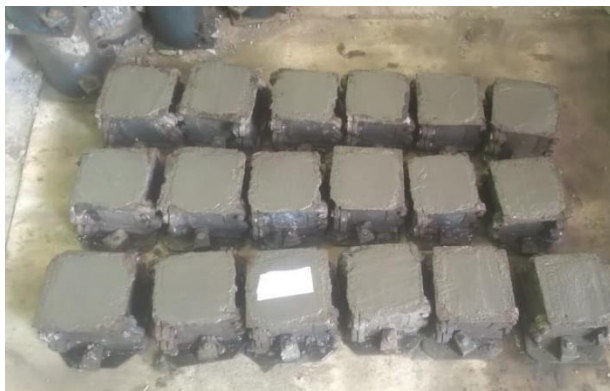
Fig. 3: Cubes (100 ×100 ×100 mm) During Casting
