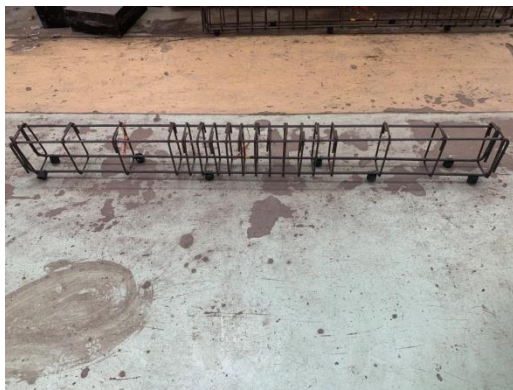
Fig.(2-a): Reinforcement detail for flexure
