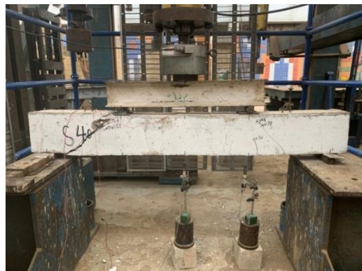
Fig.( 5-b): crack pattern- Shear
