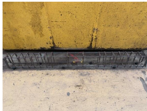
Fig.(2-b): Reinforcement detail for shear
