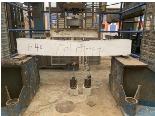
Fig.(5-a): crack pattern- Flexure
