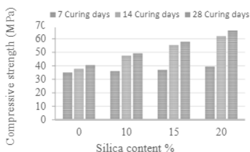
Fig6 Compressive strength for 45 percent-RCA with Silica after seven, fourteen and twenty-eight days of curing
