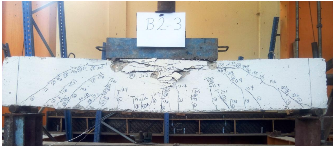
Fig. 4: Crack pattern for specimen B2-3
