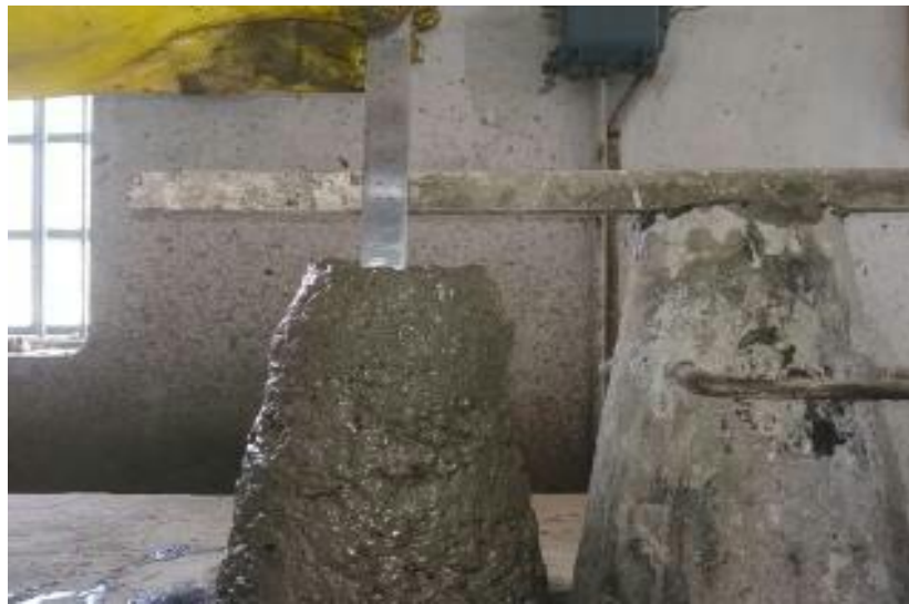
Figure 4.1 Slump cone test
