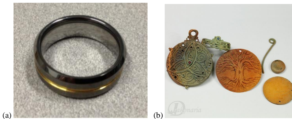
Figure 8: (a) Wedding Ring from Tungsten Carbide. (b) Jewellery from Goldie Bronze. Both sintered.[13, 27]
