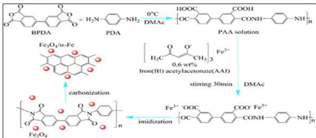
Figure no 1: the synthesis procedure for the preparation of carbon films derived from PI, PI-Fe composite film
