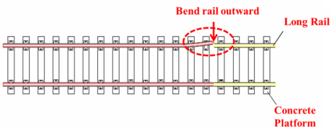
Fig 5 Dislocation of rail at one end
