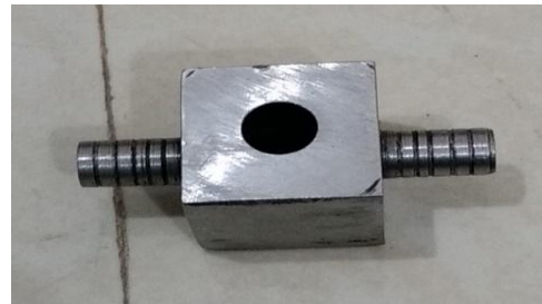
Figure.3.2 Top view of Fuel Cock make in metal
