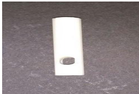
Figure.2.1 Top View of Fuel Cock makes in Rapid Prototype Machine Figure.2.2 Rod make in Rapid Prototype Machine
