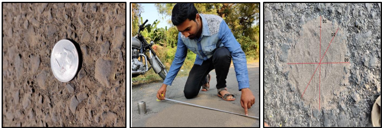
Fig.4: surface unevenness Fig.5: Sand Patch Dia. Measurement Fig.6: patch illustrating D 1 ,D 2 ,D 3
