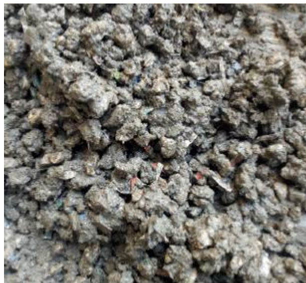
Figure 4. Tin fibers in concrete
