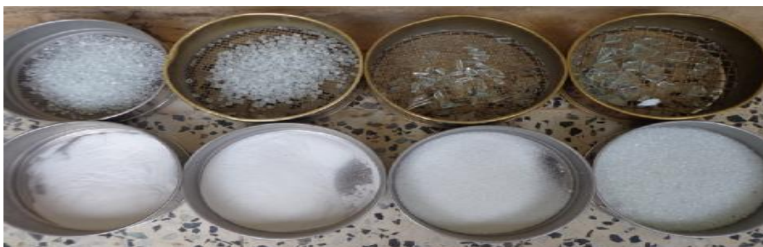
Figure (1): Particles shape of coarse WG after sieve analysis
