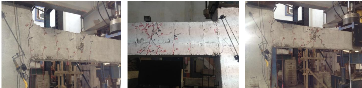
e) S5, shear failure of concrete at end of encased steel section in beam
