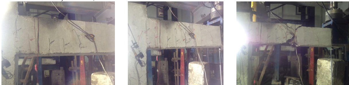
f) S6, shear failure in RC at end of encased steel section in beam
