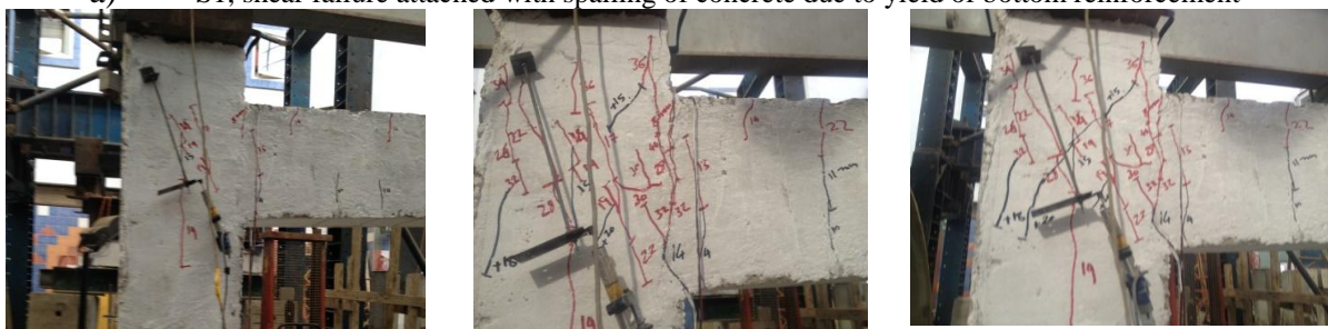
b) S2, shear failure at joint zone combined with yielding column reinforcement
