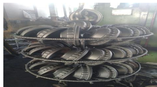
Fig 5.2: - Actual Photo of hanger during trial test(After shotBlasting)
