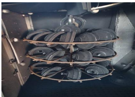
Fig 5.1: - Actual Photo of hanger during trial test(Before shot blasting).
