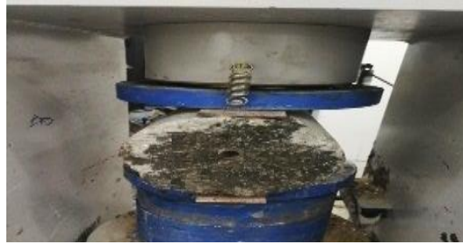
Fig.(6) Plain concrete cylinders with internal injection by epoxy.
