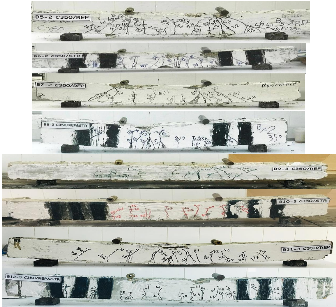
Fig:(8) Pattern of crack of beams
