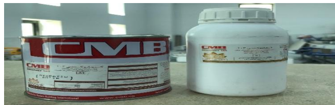
Fig (2): The Epoxy (KEMA-EPOXY103) used as internal injected material.
