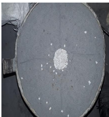
Figure 1: Stone Column embedded in pond ash
