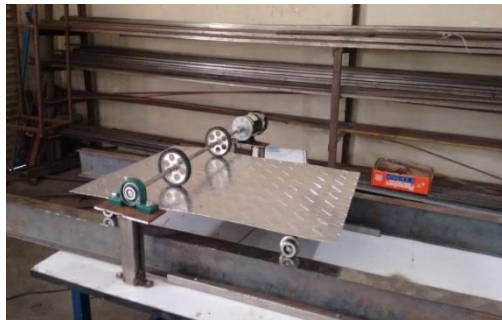
Fig. 2: Experimental setup for stage 1(I-section track)
