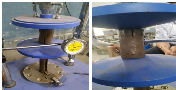
Figure 2 Soil sample during unconfined compressive strength test
