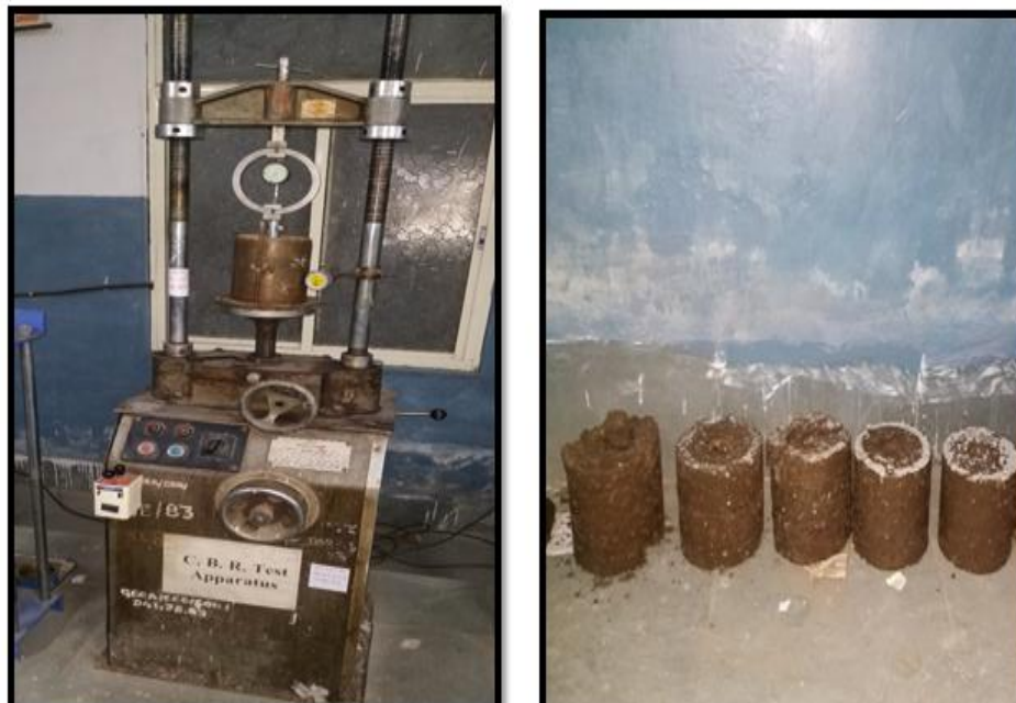
Figure 4 Soil sample of C.B.R. after test
