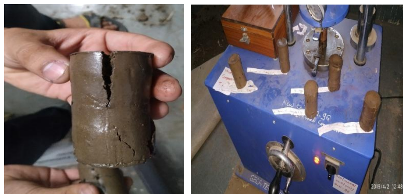
Figure 3 Soil sample after unconfined compressive strength test
