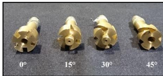
Fig. 4 A photograph of the atomizing air swirlers
