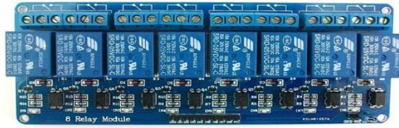
Fig. 11 Relay interface board
