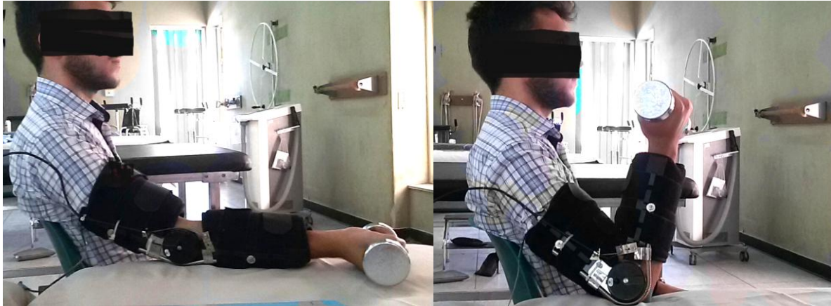
Figure 6: The device can hold the arm with different kilograms of weights.
