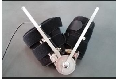
Figure 5: Using goniometer to limit the angle of the metal-arm brace.
