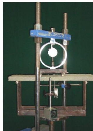
Fig.2 Flexural Test setup
