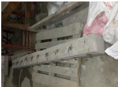
e) (P-B) After implanting shear connectors
