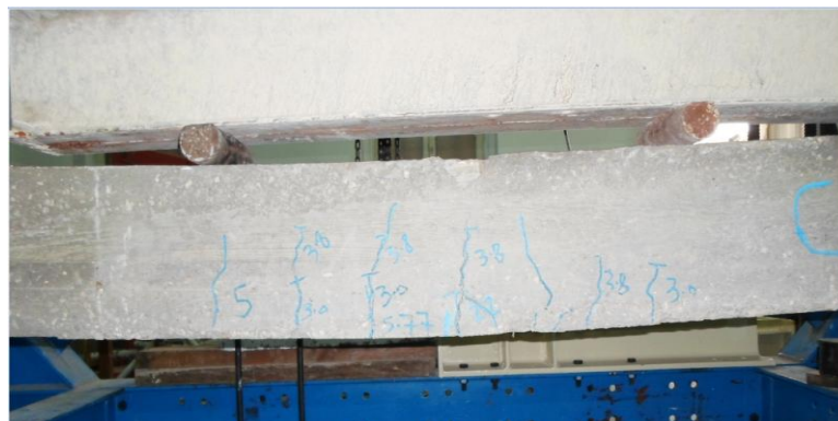
Figure 6 Control beam (C-B) cracks Pattern
