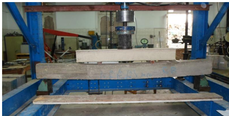
Figure 5 Control beam (C-B) Flexure failure
