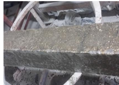
c) Akmon anchor used for fixing glass fiber sheets to R.C. Beam
