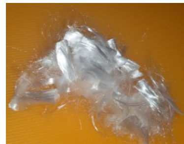
f) Polypropylene fibers used in strengthening mix.
