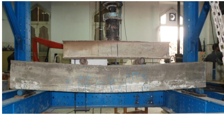
Figure 7 Strengthened beam (FE-C) Flexure failure
