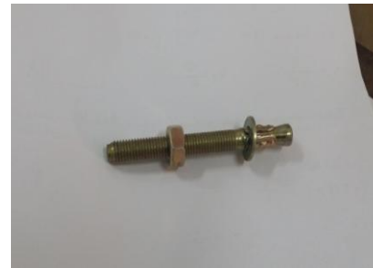
c) Akmon anchor used for fixing glass fiber sheets to R.C. Beam
