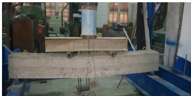
Figure 9 Strengthened beam ( P-B )Flexure failure
