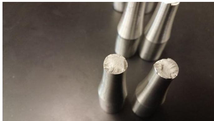
Figure 6. Failed surface of sample #1.
