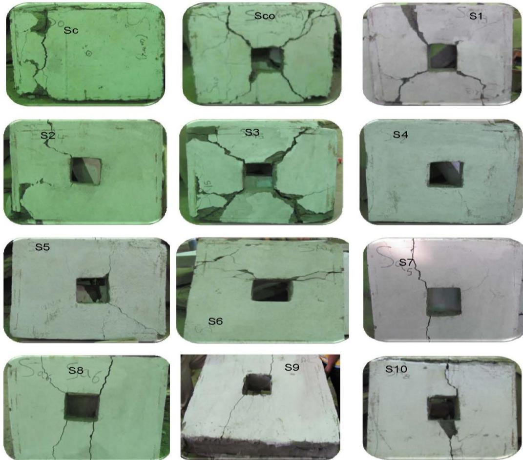
**FIGURE 10. CRACKING PATTERN OF THE TEST SPECIMENS**
