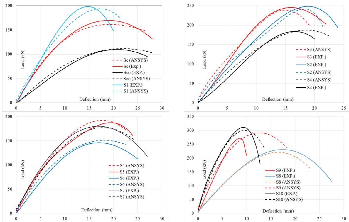
FIGURE 11. LOAD-DEFLECTION CURVES FOR EXPERIMENTAL VERSUS NUMERICAL MODELS
