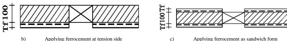
FIGURE 2. STRENGTHENING SCHEMS OF SLABS WITH FERROCEMENT
