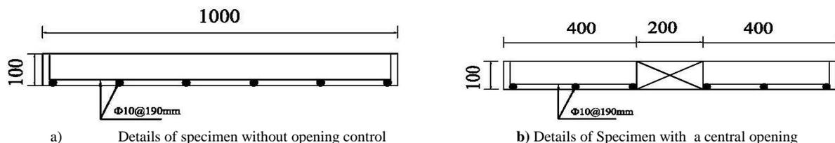
FIGURE 1. DIMENSIONS AND REINFORCEMENT DETAILS OF CONTROL SPECIMENS
