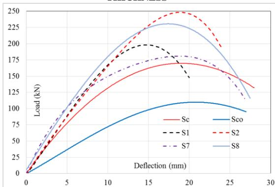
**FIGURE 8. EFFECT OF TYPE OF WIRE MESH**
