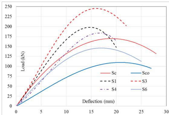
**FIGURE 6. EFFECT OF FERROCEMENT THICKNESS**
