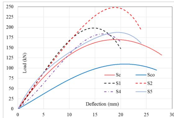
**FIGURE 7. EFFECT OF NUMBER OF WIRE MESH PER LAYER**
