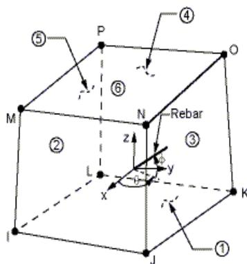
FIGURE 5.a. SOLID65 3-D REINFORCED CONCRETE SOLID ELEMENT
