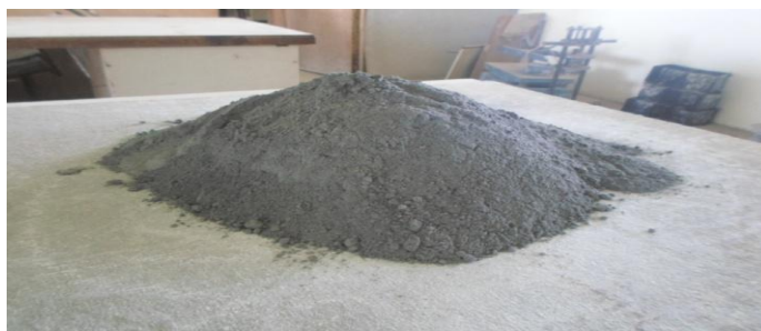
Plate 4: Pulverised Fuel Ash (Source: laboratory sample)
