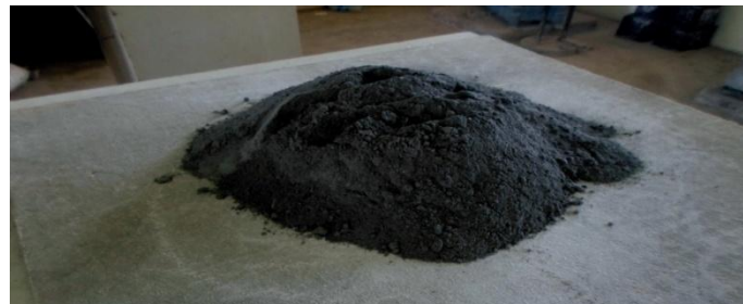
Plate 6: Quarry Dust(Source: laboratory sample)
