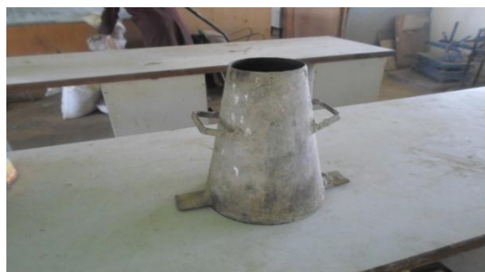
Plate 7: Slump Cone (Source: prefabricated laboratory equipment)
