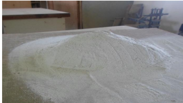
Plate 5: Carbide Waste(Source: laboratory sample)
