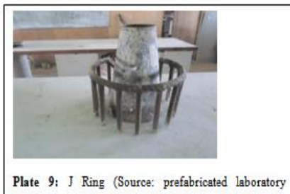
Plate 10: J Ring Test (Source: prefabricated laboratory equipment)
