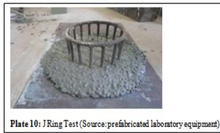
Plate 9: J Ring (Source: prefabricated laboratory equipment)
