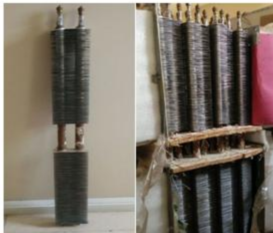
Photograph of actual finned heat pipes arranged in staggered array
